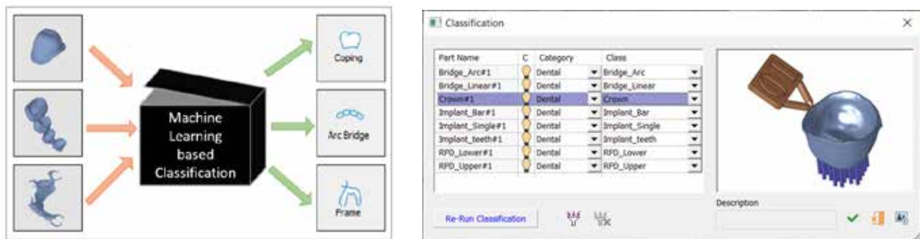
Figure 4: Part Classification using a Machine Learning Platform
